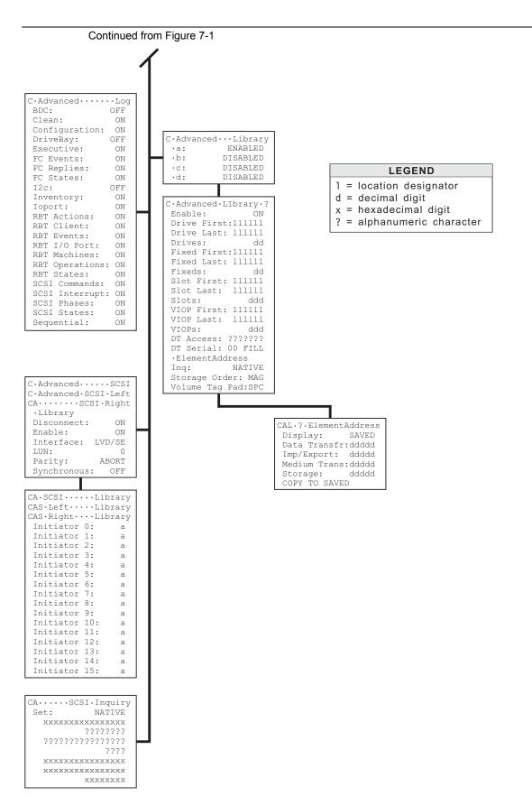
Figure 7-2 The TLS Configuration Menu (Part 2)
